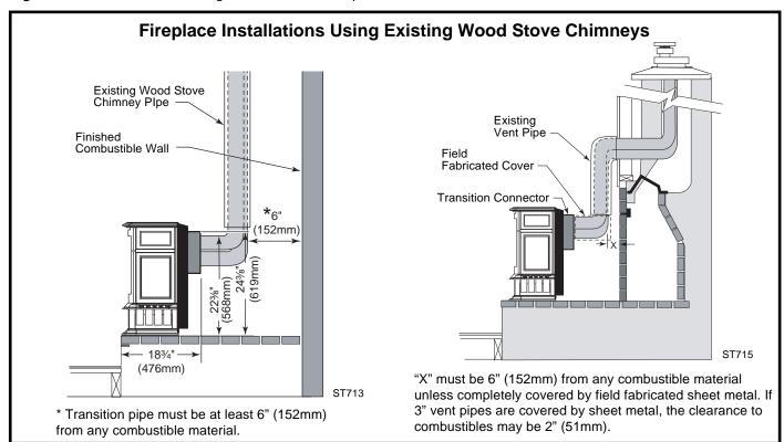
Fig. 37 PDV20 installations using existing wood stove chimney pipe.
